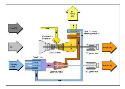
Figure 1.1: Schematic diagram illustrating the Rankine Cycle
