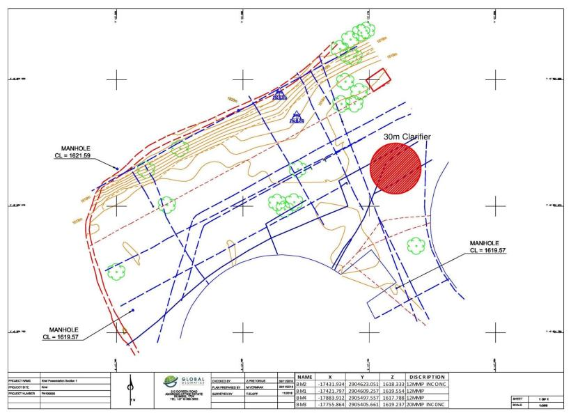
Figure 4.3: A Map illustrating the pre-existing underground piping and electrical infrastructure within the north cooling towers at the Kriel Power Station.
